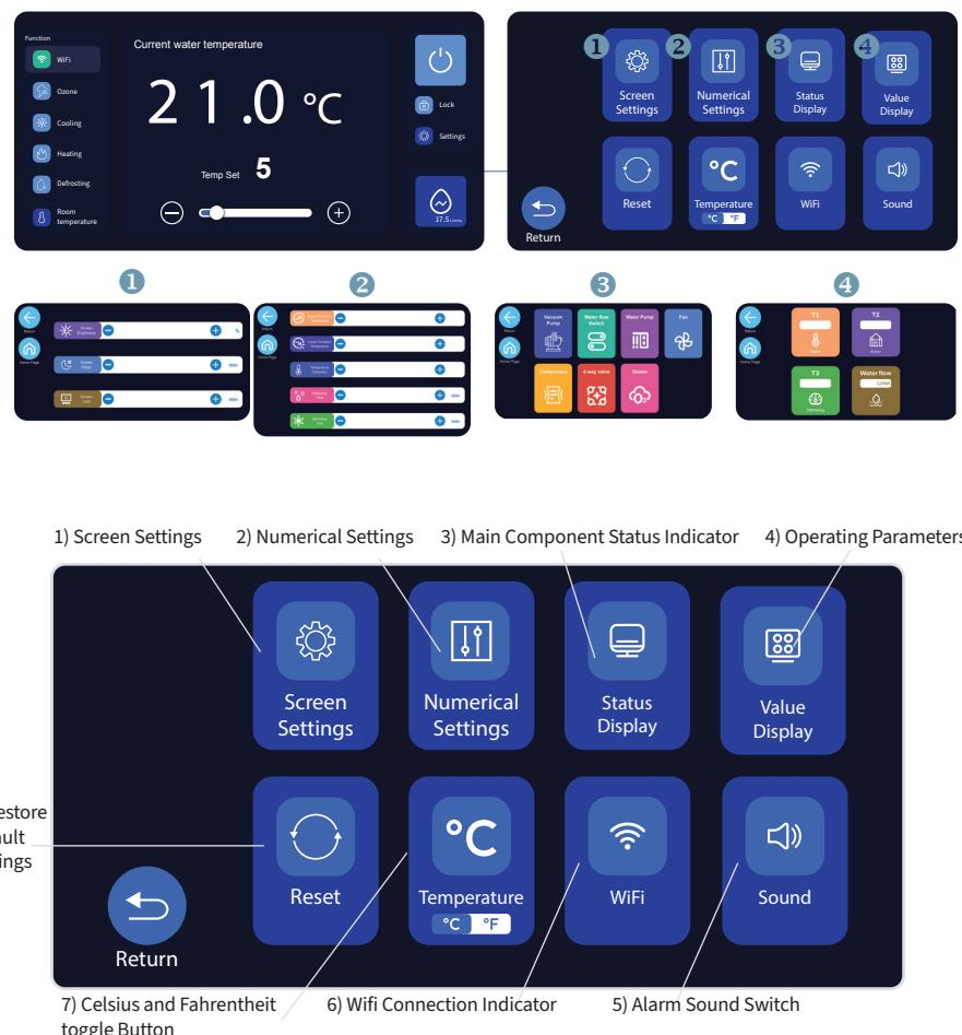
Tap the **Screen Settings** button to enter the sub-menu, where you can set the operating parameters of the main components, as shown below.
